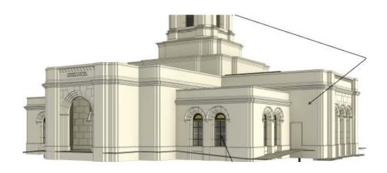
The cupola is technically a component of the steeple, but in the shape of a hip style roof, which may at first suggest that building height should consider the cupola. However, the cupola does not form the "main roof" of the building. Its size is only a small fraction of the flat roof below. As such, part "c" of the building height
