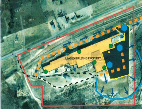
QUARRY OPERATIONS INCLUDE: GYPSUM ORE ROCK CRUSHING, SCREENING PLANT AND CONVEYANCE, LOADING OF OPEN TOP RAILCARS AND LOADING OF OPEN TOP TRAILERS
